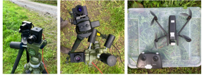
Fig. 1: Left and middle: The two different sensor setups. Right: The UAV of model Anafi from Parrot.
